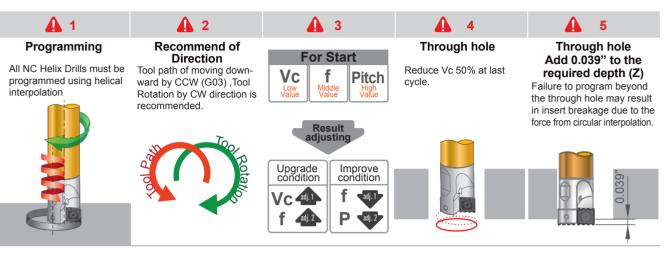
• The NC Helix Drill is programmed using "Helical interpolation" on CNC machine, the CNC controller must have 3-axis simultaneously motion function.
