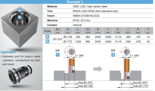
**•** Each holder "NC Helix Drill" can machine different diameters and hole depths.
